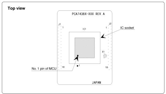
Figure 4.2 Inserting an MCU
